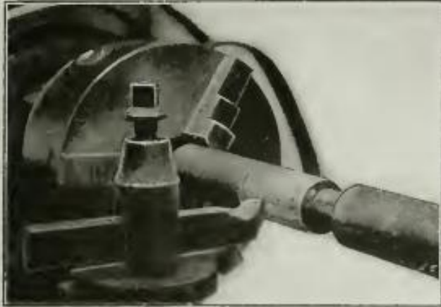
Fig. 2. Appearance of a Three-Jaw Automatic Universal Lathe Chuck. A Speedy Chuck and a Type Widely Used in All Machine Shops. The Jaws Can Be Reversed, Thus Giving a Very Wide Scope of Action.
