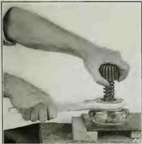
A New Cutter which Lends Itself Well to the Making of Amateur Quenched Spark Gaps.
